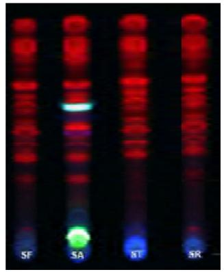
Chemical fingerprint profiles of *Sida* species on HPTLC plates detected by UV illumination.
