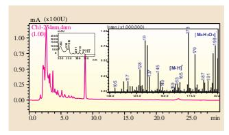
Representative HPLC chromatograms: ethylacetate extract of aerial part of *Bidens pilosa* (100mg/mL). Characteristic UV and ESI-MS mass spectra of PHT are shown in the inset of chromatogram.
