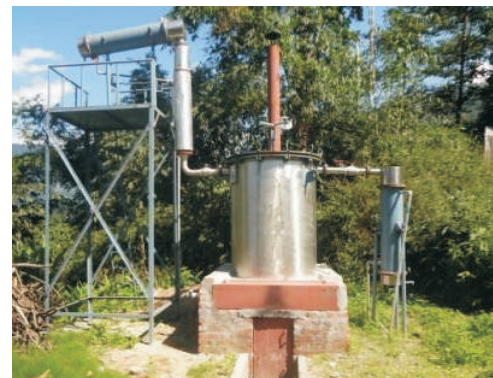
Directly fired improved distillation unit
