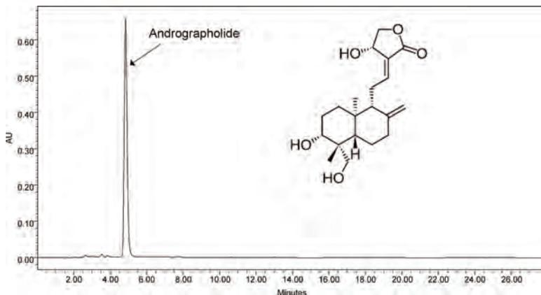
Fig: HPLC chromatogram of andrographolide (95.9%) produced on a laboratory scale
