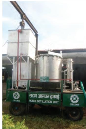
Mobile SS distillation units installed at ICAR Research Complex for NEH region
