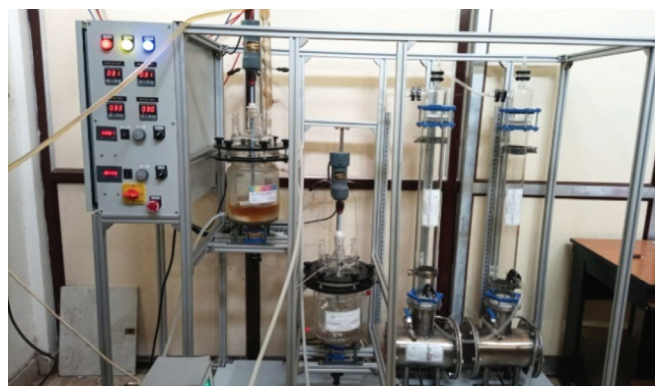
Fig. A prototype of pulse partition column system used for extraction and purification of ricinoleic acid from castor oil.
