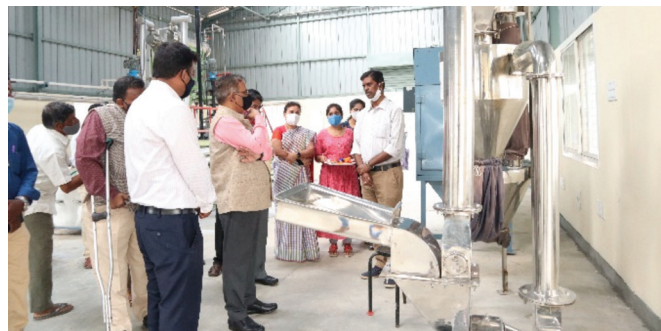
Fig. Inspection of pilot-scale primary and secondary leaf grading machines and SS-316 Pulverizer.
